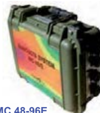
Mangusta MC 48-96E Geoelectrical Tomography Equipment
