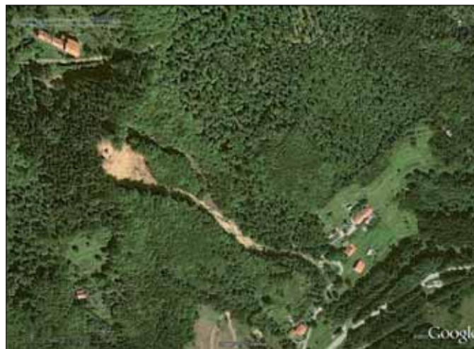
Figura 7 - Satellite view of a soil slip-debris flow near Pracchia (Pistoia Apennines).
